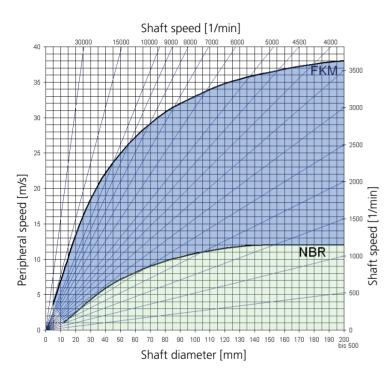
The diagram is for no-pressure operation and favourable conditions with regard to lubrication and heat dissipation (type OS-F10).
